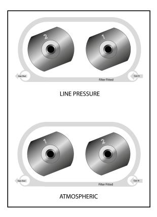
Figure 1 Interchangeable Gas Inlet/Outlet Fittings
