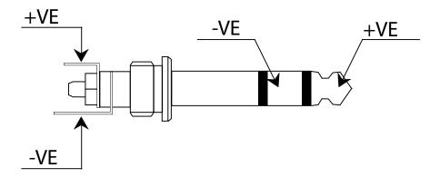
Figure 3 Jack Plug Wiring
