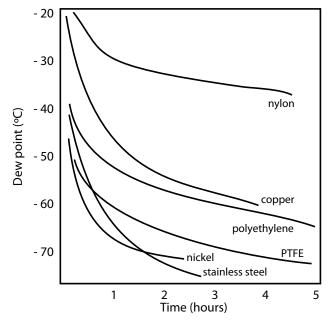
Figure 4 Material Permeability Comparison
