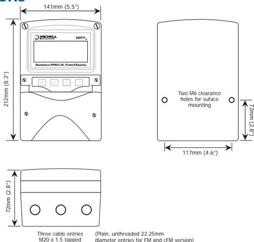
Three cable entries M20 x 1.5 tapped (Plain, unthreaded 22.25mm diameter entries for FM and cFM version)
