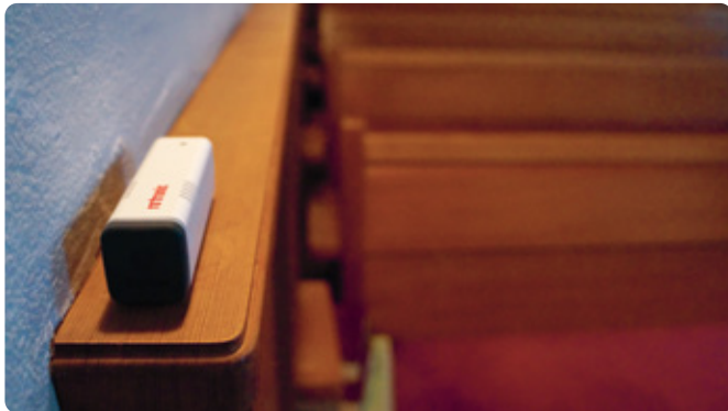
RMS wireless mini data logger records humidity and temperature.
